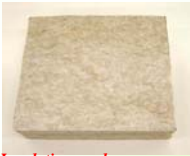
Insulation made from bamboo fiber
